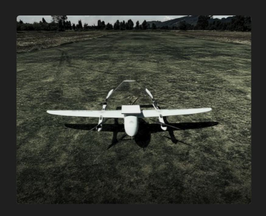
ORKID 260VTOL ISR comes equipped with full integration with Starlink's satellite constellation for real-time telemetry and video feed, without the need for expensive ground-based radio infrastructure.
